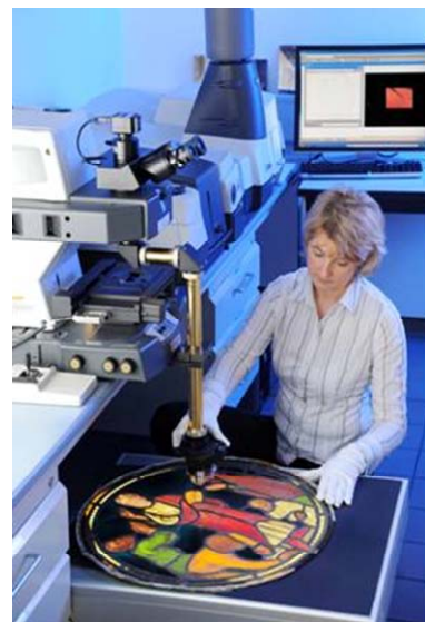
Figure 1: FTIR spectroscopy with extension arm equipment.
