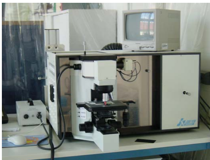
Figure 2: \mu -Raman spectroscopy.
