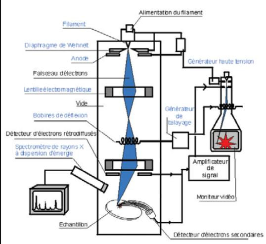
An electron beam is produced by a thermo electronic effect from a tungsten filament raised to high temperature (2700°C). This beam is accelerated by the high tension created between the filament and the anode. It is then focused on the sample by a series of three electromagnetic lenses. This probe, which is under 4 nm of diameter, scan the surface of sample point by point.
