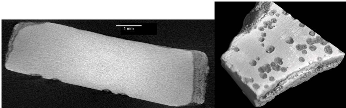
These two figures show the reconstruction of a medieval blue glass with corrosion (left and right faces) and corrosion pits (bottom). The left image is a slice; the right image is a 3D image of the same sample. (Sample courtesy of DBV Cologne, sample n° med 2)
