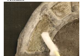
8. Final swab clean with Dichloromethane
