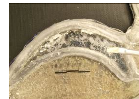
6. Remaining flakes of coating brushed off
